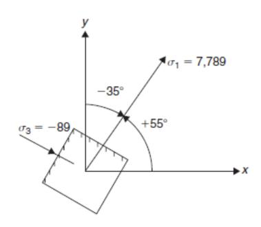
find: the magnitude and direction of the maximum shear stress and illustrate with a sketch.
