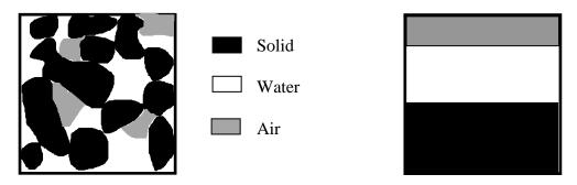
Figure 1: Air, Water and Solid phases in a typical soil
