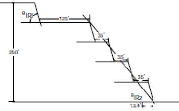
(b) Working pit slope angle measured at two spots
