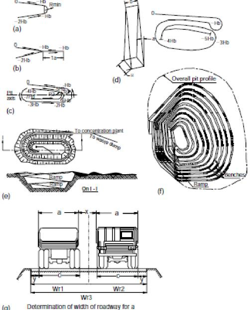
(g) Determination of width of roadway for a motor-road with one and more traffic lanes
