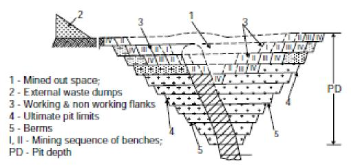
(a) For steep orebodies a suitable pit slope angle at foot wall side is also essential
