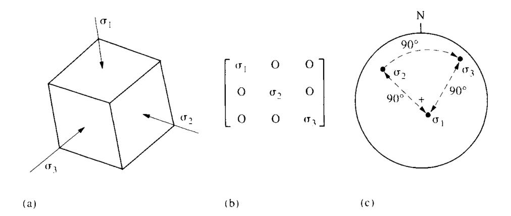
(a) Principal stresses acting on a small cube, (b) Principal stresses expressed in matrix form, (c) Principal stress orientations shown on a hemispherical projection.
