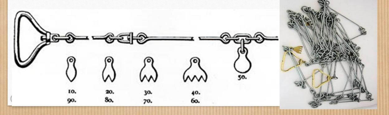
Metric Chains: Metric chains are generally available in lengths of 5, 10, 20 and 30 metres. To enable the reading of fractions of a chain without much difficulty, tallies are fixed at every metre length for chains of 5 m and 10 m lengths and at every fivemetre length for chains of 20 m and 30 m lengths.
