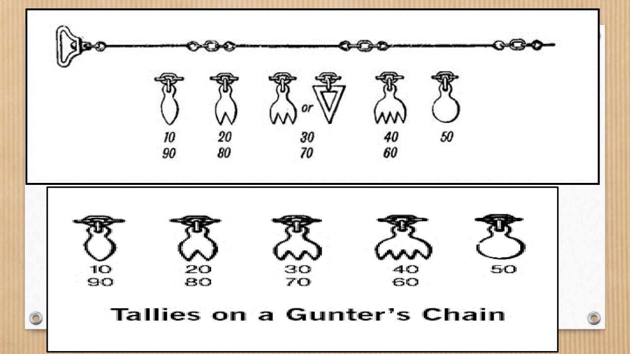
**Engineer's Chain:** The engineer's chain is 100 ft. long and consists of 100 links, each link being 1 ft. long. Tallies are provided at every 10 links, then central tally being round.
