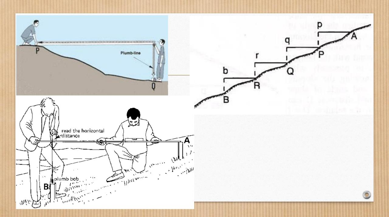
**Indirect Method:** When the slope of the ground surface is long and gentle, the stepping method is not suitable, in such a case, the horizontal distance may be measured by the following process:
