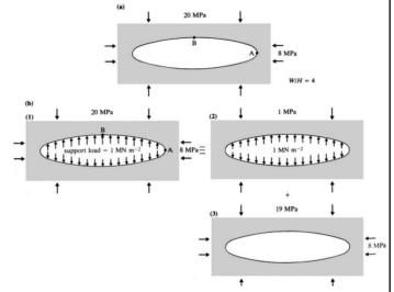
Support pressure does not significantly modify the elastic distribution around an underground opening
