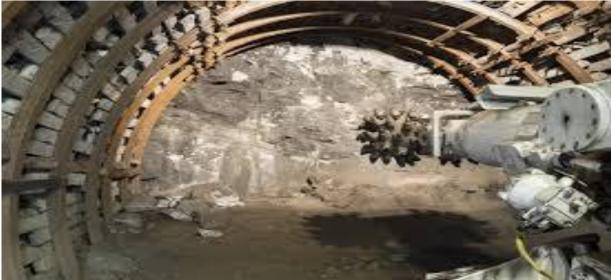
The primary opening into an underground mine to provide access for people, materials, and equipment and to enable the ore to be brought to surface can be a shaft sunk vertically or on an "incline"; a "decline," which is a ramp driven into the earth usually in a spiral fashion; or an "**adit**," which is a main horizon/main access opening.
