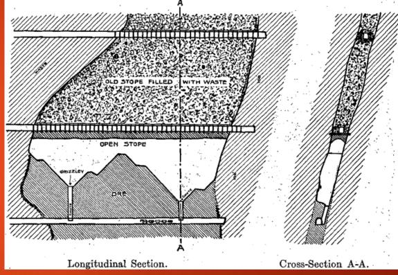
**Overhand stoping:** In overhand stoping, the deposit is worked from the bottom upward, the reverse of underhand stoping. With the advent of rock blasting and power drills, it became the predominant direction of stoping
