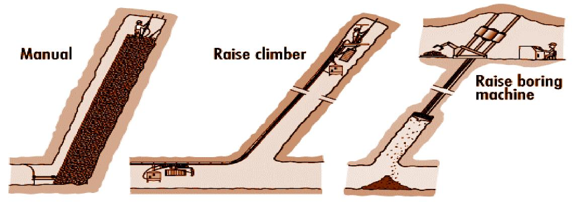
**Manual raising** is difficult, dangerous, assigned only to experienced miners in good physical condition. The raise section is divided into two compartments by a timbered wall. One is kept open for the **ladder** used for climbing to the face, air pipes, etc. The other fills with **rock** from blasting, as a **platform** when drilling the round. The work involves ladder climbing, timbering, rock drilling and blasting and blasting and blasting and blasting of the properties of the p
