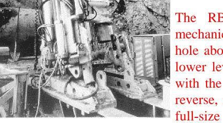
The RBM is a powerful machine that breaks the rock mechanically. It is erected on top of the planned raise and a pilot hole about 300 mm in diameter is drilled to break through at a lower level target. The pilot drill is replaced by a reamer head with the diameter of the intended raise and the RBM is put in reverse, rotating and pulling the reamer head upward to create a full-size circular raise.
