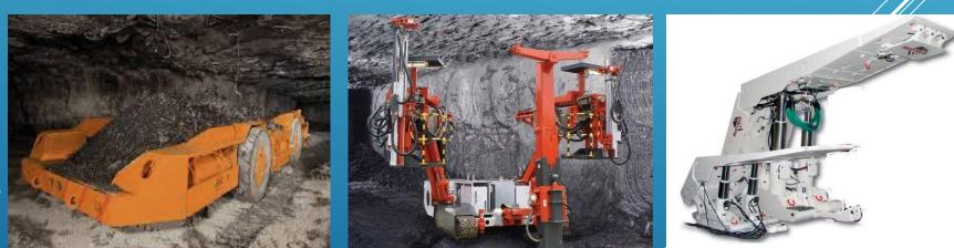
Drilling machines, road header, shearer, continuous miner, side discharge loader, Load haul dump
